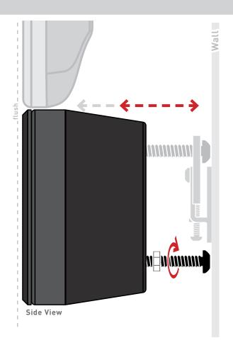
Adjust **Mounting Bolts** to align Speaker flush with TV
