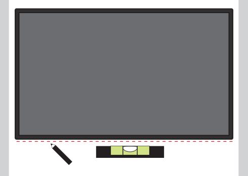
Mount **TV** level to wall and draw **Guide Line** level with TV edge\*
