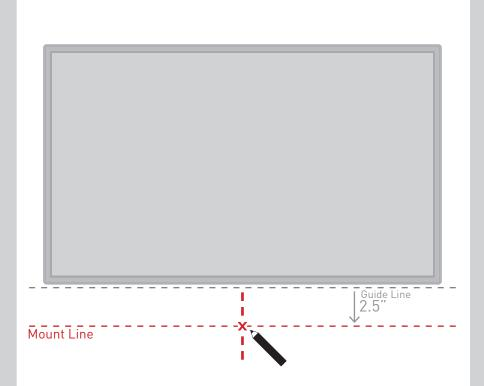
Draw a second **Mount Line** 2.5" from **Guide Line**Find **Center** of TV and **Mark** on **Mount Line**
