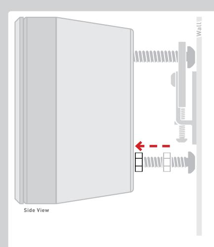
Adjust Lock Nuts to secure assembly
