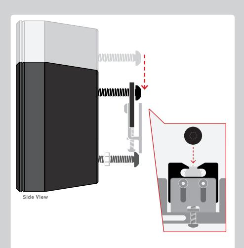
Hang speaker by securing **Top Mounting Bolts** in **Mounting Plates**
