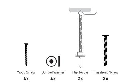
NOTE: Not all parts in the Wall Mount Kit will be used during install
