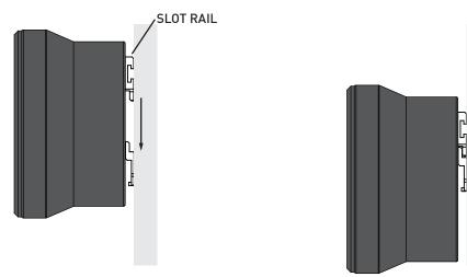
Remove the **TEMPLATE** and connect wiring to speaker. Mount speaker by sliding the **SLOT RAILS** (located on the back of the speaker) over the **WALL PLATES**. Minor adjustments can be made by sliding the speaker horizontally or shifting the **WALL PLATES** vertically.
