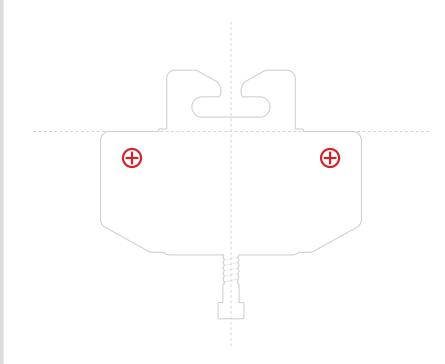
Remove **Brackets** and drill\* **Pilot Holes** at mark locations for **Wood Screws** or **Drywall Anchors**
