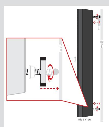
Extend bottom **T-Bar Bolts** to wall and adjust to align Speaker flush with TV
