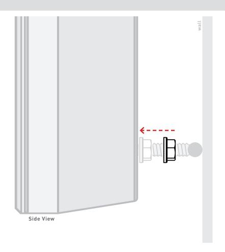
Adjust **Lock Nuts** to secure T-Bar Bolts
