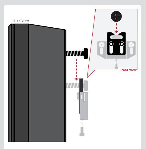
Hang speakers by securing **Mounting Bolts** in **Brackets**
