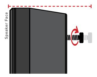
Measure depth from face of TV to the Wall and adjust speaker **Mounting Bolts** to match
