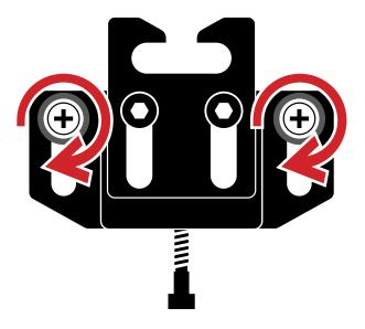
Remove **Templates** and attach **Brackets** to wall with **Wood Screws** or **Drywall Anchors**
