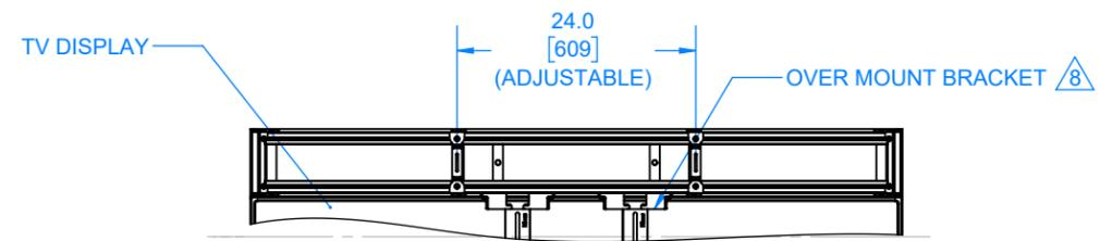
BACK VIEW WITH OVER MOUNT BRACKET SCALE 1 : 20
