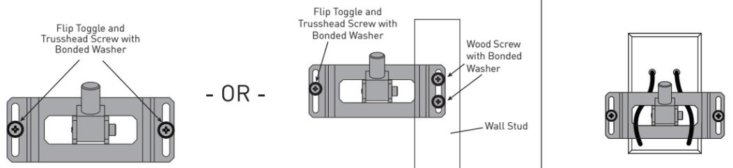
The **BRACKET PLATE** can mount over a wall plate. Speaker wires can thread through **BRACKET PLATE** holes.
